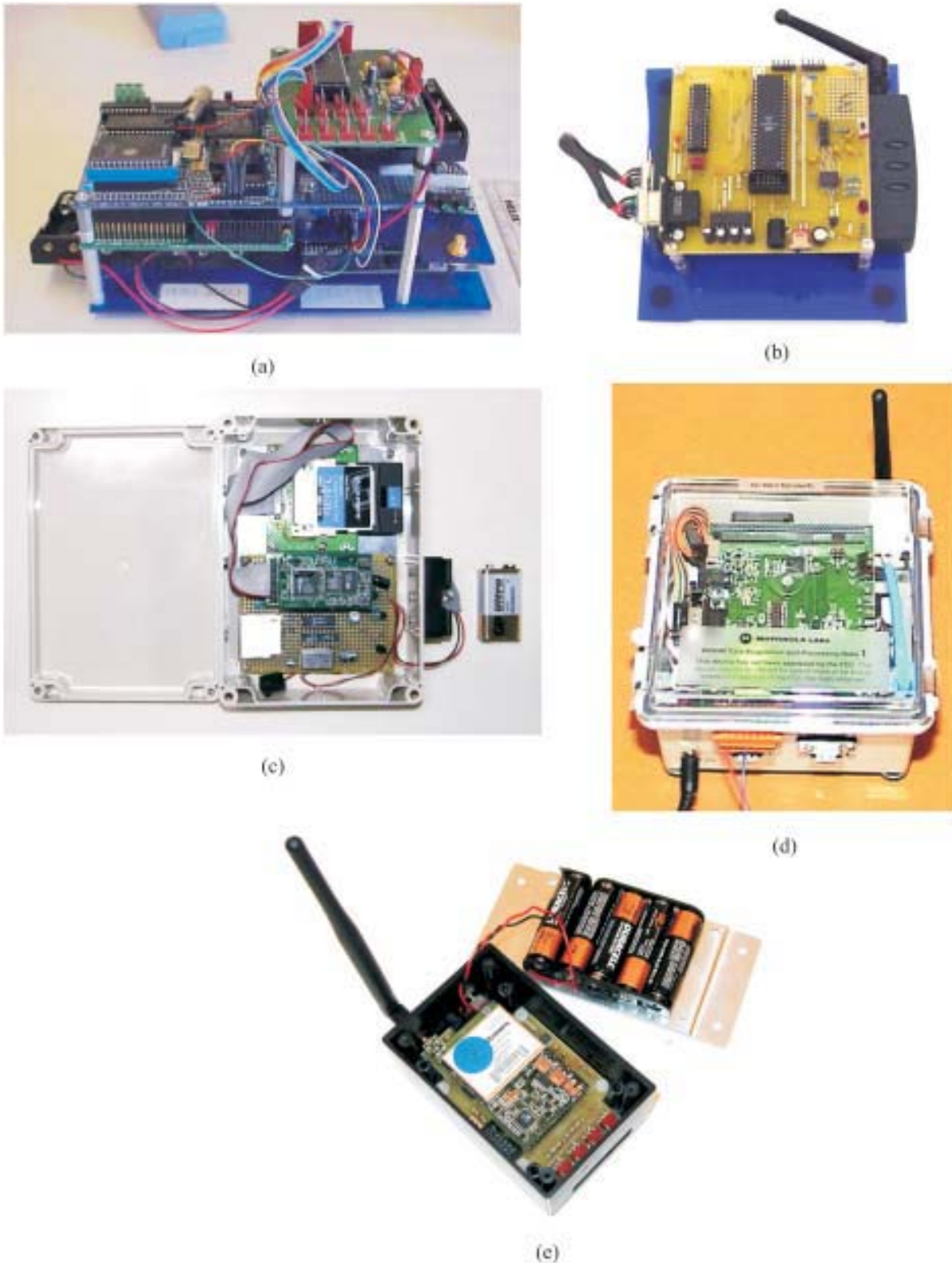
Figure 3. Academic wireless sensor prototypes: (a) WiMMS wireless sensor (Straser and Kiremidjian, 1998); (b) dual-core prototype by Lynch (2002); (c) RIMS wireless sensor based on Aoki et al. (2003); (d) Husky wireless sensor (Allen, 2004; courtesy of Motorola Labs); (e) wireless sensor prototype by Wang et al. (2005).
